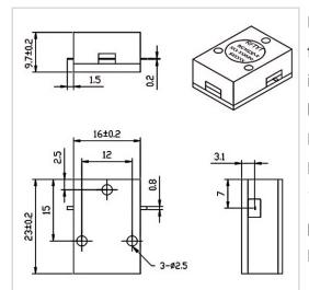
RF Solution offer a wide selection of Drop in Isolator for global customers. WG1623D is a Drop in Isolator in Frequency Range of 5.0~7.3 GHz. It is made of high quality materials under a high standard, the Bandwidth Max of this product is 100%, Insertion Loss Max is 0.30~0.60 dB and Isolation Min is 18.0~23.0 dB. The component has a good working performance and stability, it is ideal for handling a Forward Power of 30 W.
