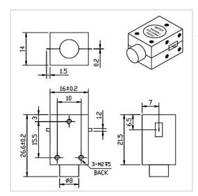
RF Solution offer a wide selection of Drop in Isolator for global customers. WG1622B is a Drop in Isolator in Frequency Range of 6.0~18.0 GHz. It is made of high quality materials under a high standard, the Bandwidth Max of this product is 100%, Insertion Loss Max is 0.60~1.50 dB and Isolation Min is 10.0~20.0 dB. The component has a good working performance and stability, it is ideal for handling a Forward Power of 30 W.
