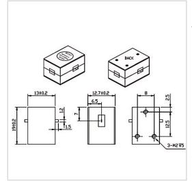
RF Solution offer a wide selection of Drop in Isolator for global customers. WG1319C is a Drop in Isolator in Frequency Range of 6.0~12.0 GHz. It is made of high quality materials under a high standard, the Bandwidth Max of this product is 40%, Insertion Loss Max is 0.30~0.60 dB and Isolation Min is 16.0~23.0 dB. The component has a good working performance and stability, it is ideal for handling a Forward Power of 30 W.
