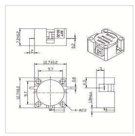
RF Solution offer a wide selection of Drop in Isolator for global customers. WG1313T is a Drop in Isolator in Frequency Range of 800~7000 MHz. It is made of high quality materials under a high standard, the Bandwidth Max of this product is 25%, Insertion Loss Max is 0.30~0.50 dB and Isolation Min is 18.0~23.0 dB. The component has a good working performance and stability, it is ideal for handling a Forward Power of 60 W.
