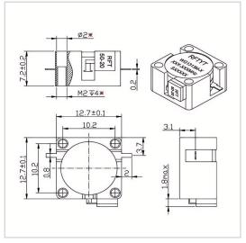
RF Solution offer a wide selection of Drop in Isolator for global customers. WG1313M is a Drop in Isolator in Frequency Range of 800~7000 MHz. It is made of high quality materials under a high standard, the Bandwidth Max of this product is 25%, Insertion Loss Max is 0.30~0.50 dB and Isolation Min is 18.0~23.0 dB. The component has a good working performance and stability, it is ideal for handling a Forward Power of 60 W.
