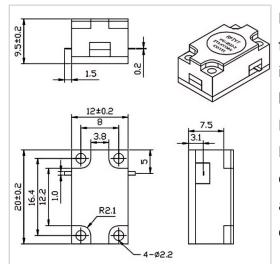
RF Solution offer a wide selection of Drop in Isolator for global customers. WG1220D is a Drop in Isolator in Frequency Range of 5.5~7.0 GHz. It is made of high quality materials under a high standard, the Bandwidth Max of this product is 20%, Insertion Loss Max is 0.30~0.50 dB and Isolation Min is 18.0~23.0 dB. The component has a good working performance and stability, it is ideal for handling a Forward Power of 30 W.
