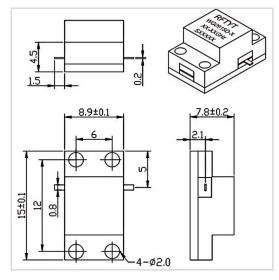
RF Solution offer a wide selection of Drop in Isolator for global customers. WG0915D is a Drop in Isolator in Frequency Range of 6.0~18.0 GHz. It is made of high quality materials under a high standard, the Bandwidth Max of this product is 40%, Insertion Loss Max is 0.30~0.60 dB and Isolation Min is 18.0~23.0 dB. The component has a good working performance and stability, it is ideal for handling a Forward Power of 30 W.
