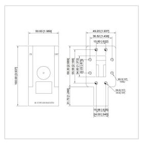
RF Solution offer a wide selection of Waveguide Isolator for global customers. UIYWI49100A is a Waveguide Isolator in Frequency Range of 5.4~8.0 GHz. It is made of high quality materials under a high standard, the Bandwidth Max of this product is 20%, Insertion Loss Max is 0.25~0.40 dB and Isolation Min is 18.0~25.0 dB. The component has a good working performance and stability, it is ideal for handling a Forward Power of 100 W.
