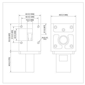
RF Solution offer a wide selection of Waveguide Isolator for global customers. UIYWI4893A is a Waveguide Isolator in Frequency Range of 8.0~12.0 GHz. It is made of high quality materials under a high standard, the Bandwidth Max of this product is 100%, Insertion Loss Max is 0.50 dB and Isolation Min is 18.0 dB. The component has a good working performance and stability, it is ideal for handling a Forward Power of 100 W.
