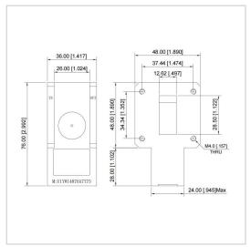
RF Solution offer a wide selection of Waveguide Isolator for global customers. UIYWI4876A is a Waveguide Isolator in Frequency Range of 7.0~10.0 GHz. It is made of high quality materials under a high standard, the Bandwidth Max of this product is 20%, Insertion Loss Max is 0.25~0.40 dB and Isolation Min is 20.0~25.0 dB. The component has a good working performance and stability, it is ideal for handling a Forward Power of 100 W.
