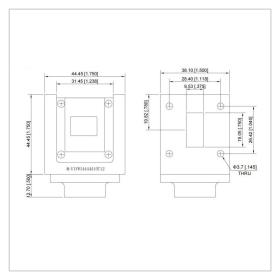
RF Solution offer a wide selection of Waveguide Isolator for global customers. UIYWI4444A is a Waveguide Isolator in Frequency Range of 10.0~15.0 GHz. It is made of high quality materials under a high standard, the Bandwidth Max of this product is 20%, Insertion Loss Max is 0.30~0.35 dB and Isolation Min is 20.0~23.0 dB. The component has a good working performance and stability, it is ideal for handling a Forward Power of 100 W.
