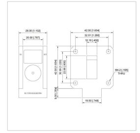
RF Solution offer a wide selection of Waveguide Isolator for global customers. UIYWI4242A is a Waveguide Isolator in Frequency Range of 8.0~12.4 GHz. It is made of high quality materials under a high standard, the Bandwidth Max of this product is 25%, Insertion Loss Max is 0.25~0.50 dB and Isolation Min is 18.0~23.0 dB. The component has a good working performance and stability, it is ideal for handling a Forward Power of 100 W.
