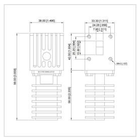
RF Solution offer a wide selection of Waveguide Isolator for global customers. UIYWI3898A is a Waveguide Isolator in Frequency Range of 12.0~18.0 GHz. It is made of high quality materials under a high standard, the Bandwidth Max of this product is 100%, Insertion Loss Max is 0.40 dB and Isolation Min is 20.0 dB. The component has a good working performance and stability, it is ideal for handling a Forward Power of 100 W.
