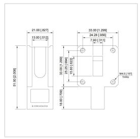
RF Solution offer a wide selection of Waveguide Isolator for global customers. UIYWI3333A is a Waveguide Isolator in Frequency Range of 12.4~18.0 GHz. It is made of high quality materials under a high standard, the Bandwidth Max of this product is 20%, Insertion Loss Max is 0.30~0.35 dB and Isolation Min is 20.0~23.0 dB. The component has a good working performance and stability, it is ideal for handling a Forward Power of 100 W.
