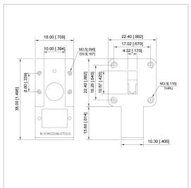
RF Solution offer a wide selection of Waveguide Isolator for global customers. UIYWI2238A is a Waveguide Isolator in Frequency Range of 17.7~21.6 GHz. It is made of high quality materials under a high standard, the Bandwidth Max of this product is 90%, Insertion Loss Max is 0.30dB and Isolation Min is 20.0 dB. The component has a good working performance and stability, it is ideal for handling a Forward Power of 30 W.
