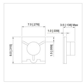
RF Solution offer a wide selection of Microstrip Isolator for global customers. UIYMI78A is a Microstrip Isolator in Frequency Range of 7.0~12.0 GHz. It is made of high quality materials under a high standard, the Bandwidth Max of this product is 40%, Insertion Loss Max is 0.50~0.60 dB and Isolation Min is 18.0~20.0 dB. The component has a good working performance and stability, it is ideal for handling a Forward Power of 15 W.
