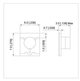
RF Solution offer a wide selection of Microstrip Isolator for global customers. UIYMI67A is a Microstrip Isolator in Frequency Range of 8.0~18.0 GHz. It is made of high quality materials under a high standard, the Bandwidth Max of this product is 45%, Insertion Loss Max is 0.50~0.90 dB and Isolation Min is 12.0~20 dB. The component has a good working performance and stability, it is ideal for handling a Forward Power of 15 W.
