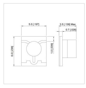
RF Solution offer a wide selection of Microstrip Isolator for global customers. UIYMI56A is a Microstrip Isolator in Frequency Range of 14.0~40.0 GHz. It is made of high quality materials under a high standard, the Bandwidth Max of this product is 20%, Insertion Loss Max is 0.50~0.70 dB and Isolation Min is 18.0~20.0 dB. The component has a good working performance and stability, it is ideal for handling a Forward Power of 10 W.
