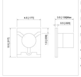
RF Solution offer a wide selection of Microstrip Isolator for global customers. UIYMI45B is a Microstrip Isolator in Frequency Range of 22.0~32.0 GHz. It is made of high quality materials under a high standard, the Bandwidth Max of this product is 25%, Insertion Loss Max is 0.7 dB and Isolation Min is 17.0 dB. The component has a good working performance and stability, it is ideal for handling a Forward Power of 2 W.
