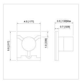
RF Solution offer a wide selection of Microstrip Isolator for global customers. UIYMI45A is a Microstrip Isolator in Frequency Range of  $18.0\sim22.0$  GHz. It is made of high quality materials under a high standard, the Bandwidth Max of this product is 20%, Insertion Loss Max is 0.6 dB and Isolation Min is 17.0 dB. The component has a good working performance and stability, it is ideal for handling a Forward Power of 2 W.
