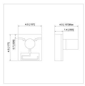
RF Solution offer a wide selection of Microstrip Isolator for global customers. UIYMI44C is a Microstrip Isolator in Frequency Range of 37.0~43.0 GHz. It is made of high quality materials under a high standard, the Bandwidth Max of this product is 100%, Insertion Loss Max is 1.4 dB and Isolation Min is 14.0 dB. The component has a good working performance and stability, it is ideal for handling a Forward Power of 2 W.
