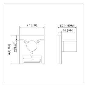
RF Solution offer a wide selection of Microstrip Isolator for global customers. UIYMI44B is a Microstrip Isolator in Frequency Range of 24.0~40.0 GHz. It is made of high quality materials under a high standard, the Bandwidth Max of this product is 15%, Insertion Loss Max is 0.7~0.90 dB and Isolation Min is 15.0 dB. The component has a good working performance and stability, it is ideal for handling a Forward Power of 15 W.
