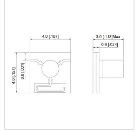
RF Solution offer a wide selection of Microstrip Isolator for global customers. UIYMI44A is a Microstrip Isolator in Frequency Range of 24.0~40.0 GHz. It is made of high quality materials under a high standard, the Bandwidth Max of this product is 15%, Insertion Loss Max is 0.7~0.90 dB and Isolation Min is 15.0 dB. The component has a good working performance and stability, it is ideal for handling a Forward Power of 15 W.
