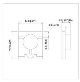
RF Solution offer a wide selection of Microstrip Isolator for global customers. UIYMI1416A is a Microstrip Isolator in Frequency Range of 2.7~4.9 GHz. It is made of high quality materials under a high standard, the Bandwidth Max of this product is 40%, Insertion Loss Max is 0.40~0.80 dB and Isolation Min is 15.0~20.0 dB. The component has a good working performance and stability, it is ideal for handling a Forward Power of 15 W.
