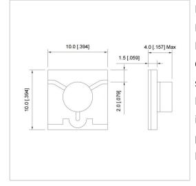
RF Solution offer a wide selection of Microstrip Isolator for global customers. UIYMI1010A is a Microstrip Isolator in Frequency Range of 5.0~8.0 GHz. It is made of high quality materials under a high standard, the Bandwidth Max of this product is 45%, Insertion Loss Max is 0.40~0.90 dB and Isolation Min is 16.0~20.0 dB. The component has a good working performance and stability, it is ideal for handling a Forward Power of 15 W.
