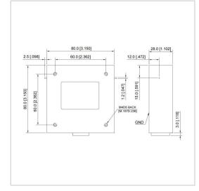
RF Solution offer a wide selection of Drop in Isolator for global customers. UIYDI8080A is a Drop in Isolator in Frequency Range of 10~55 MHz. It is made of high quality materials under a high standard, the Bandwidth Max of this product is 20%, Insertion Loss Max is 1.20~5.00 dB and Isolation Min is 11.0~20.0 dB. The component has a good working performance and stability, it is ideal for handling a Forward Power of 50 W.
