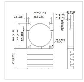
RF Solution offer a wide selection of Drop in Isolator for global customers. UIYDI80140B is a Drop in Isolator in Frequency Range of 60~200 MHz. It is made of high quality materials under a high standard, the Bandwidth Max of this product is 20%, Insertion Loss Max is 0.20~1.50 dB and Isolation Min is 18.0~25.0 dB. The component has a good working performance and stability, it is ideal for handling a Forward Power of 500 W.
