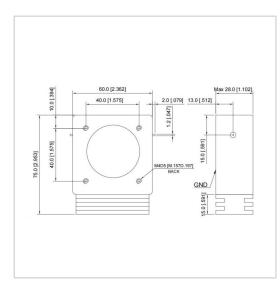
RF Solution offer a wide selection of Drop in Isolator for global customers. UIYDI6075A is a Drop in Isolator in Frequency Range of 45~270 MHz. It is made of high quality materials under a high standard, the Bandwidth Max of this product is 40%, Insertion Loss Max is 0.50~1.80 dB and Isolation Min is 18.0~23.0 dB. The component has a good working performance and stability, it is ideal for handling a Forward Power of 100/150/200 W.
