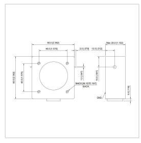
RF Solution offer a wide selection of Drop in Isolator for global customers. UIYDI6060A is a Drop in Isolator in Frequency Range of  $45\sim270$  MHz. It is made of high quality materials under a high standard, the Bandwidth Max of this product is 40%, Insertion Loss Max is  $0.50\sim1.80$  dB and Isolation Min is  $18.0\sim23.0$  dB. The component has a good working performance and stability, it is ideal for handling a Forward Power of 100/200 W.
