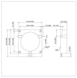
RF Solution offer a wide selection of Drop in Isolator for global customers. UIYDI5663A is a Drop in Isolator in Frequency Range of 130~900 MHz. It is made of high quality materials under a high standard, the Bandwidth Max of this product is 40%, Insertion Loss Max is 0.40~0.70 dB and Isolation Min is 16.0~23.0 dB. The component has a good working performance and stability, it is ideal for handling a Forward Power of 300 W.
