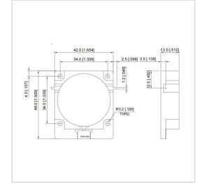
RF Solution offer a wide selection of Drop in Isolator for global customers. UIYDI4249A is a Drop in Isolator in Frequency Range of 200~1300 MHz. It is made of high quality materials under a high standard, the Bandwidth Max of this product is 35%, Insertion Loss Max is 0.25~0.65 dB and Isolation Min is 16.0~25.0 dB. The component has a good working performance and stability, it is ideal for handling a Forward Power of 100/300 W.
