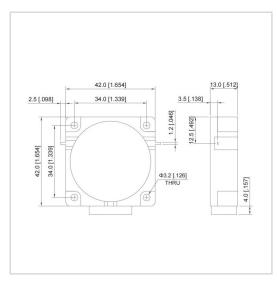
RF Solution offer a wide selection of Drop in Isolator for global customers. UIYDI4242A is a Drop in Isolator in Frequency Range of  $200{\sim}1300$  MHz. It is made of high quality materials under a high standard, the Bandwidth Max of this product is 35%, Insertion Loss Max is  $0.25{\sim}0.65$  dB and Isolation Min is  $16.0{\sim}25.0$  dB. The component has a good working performance and stability, it is ideal for handling a Forward Power of 100/300 W.
