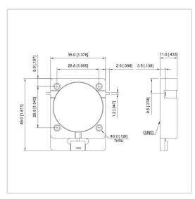
RF Solution offer a wide selection of Drop in Isolator for global customers. UIYDI3546A is a Drop in Isolator in Frequency Range of 200~1875 MHz. It is made of high quality materials under a high standard, the Bandwidth Max of this product is 40%, Insertion Loss Max is 0.20~0.65 dB and Isolation Min is 15.0~30.0 dB. The component has a good working performance and stability, it is ideal for handling a Forward Power of 300 W.
