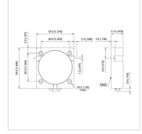
RF Solution offer a wide selection of Drop in Isolator for global customers. UIYDI3538A is a Drop in Isolator in Frequency Range of 200~1875 MHz. It is made of high quality materials under a high standard, the Bandwidth Max of this product is 40%, Insertion Loss Max is 0.20~0.65 dB and Isolation Min is 15.0~30.0 dB. The component has a good working performance and stability, it is ideal for handling a Forward Power of 300 W.
