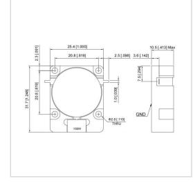
RF Solution offer a wide selection of Drop in Isolator for global customers. UIYDI2531A is a Drop in Isolator in Frequency Range of 200~3600 MHz. It is made of high quality materials under a high standard, the Bandwidth Max of this product is 30%, Insertion Loss Max is 0.20~0.60 dB and Isolation Min is 15.0~25.0 dB. The component has a good working performance and stability, it is ideal for handling a Forward Power of 200 W.
