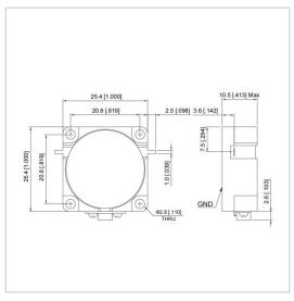
RF Solution offer a wide selection of Drop in Isolator for global customers. UIYDI2525A is a Drop in Isolator in Frequency Range of 200~3600 MHz. It is made of high quality materials under a high standard, the Bandwidth Max of this product is 30%, Insertion Loss Max is 0.20~0.60 dB and Isolation Min is 15.0~25.0 dB. The component has a good working performance and stability, it is ideal for handling a Forward Power of 200 W.
