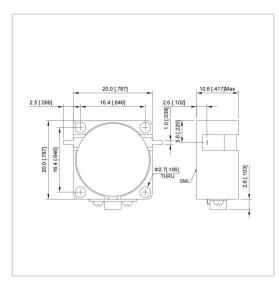
RF Solution offer a wide selection of Drop in Isolator for global customers. UIYDI2020A is a Drop in Isolator in Frequency Range of 400~3000 MHz. It is made of high quality materials under a high standard, the Bandwidth Max of this product is 30%, Insertion Loss Max is 0.25~0.70 dB and Isolation Min is 16.0~25.0 dB. The component has a good working performance and stability, it is ideal for handling a Forward Power of 100 W.
