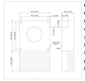
RF Solution offer a wide selection of Drop in Isolator for global customers. UIYDI100166A is a Drop in Isolator in Frequency Range of 70~900 MHz. It is made of high quality materials under a high standard, the Bandwidth Max of this product is 20%, Insertion Loss Max is 0.80~1.20 dB and Isolation Min is 16.0~17.0 dB. The component has a good working performance and stability, it is ideal for handling a Forward Power of 300/500 W.
