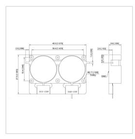
RF Solution offer a wide selection of Dual Junction Isolator for global customers. UIYDDI4027A is a Dual Junction Isolator in Frequency Range of 400~3000 MHz. It is made of high quality materials under a high standard, the Bandwidth Max of this product is 30%, Insertion Loss Max is 0.50~1.40 dB and Isolation Min is 32.0~50.0 dB. The component has a good working performance and stability, it is ideal for handling a Forward Power of 100 W.
