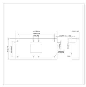
RF Solution offer a wide selection of Dual Junction Isolator for global customers. UIYDDI16080A is a Dual Junction Isolator in Frequency Range of 10~55 MHz. It is made of high quality materials under a high standard, the Bandwidth Max of this product is 20%, Insertion Loss Max is 2.40~7.00 dB and Isolation Min is 24.0~40.0 dB. The component has a good working performance and stability, it is ideal for handling a Forward Power of 50 W.
