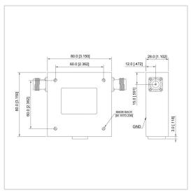
RF Solution offer a wide selection of Coaxial Isolator for global customers. UIYCI8080A is a Coaxial Isolator in Frequency Range of 10~55 MHz. It is made of high quality materials under a high standard, the Bandwidth Max of this product is 20%, Insertion Loss Max is 1.20~5.00 dB and Isolation Min is 11.0~20.0 dB. The component has a good working performance and stability, it is ideal for handling a Forward Power of 50 W.
