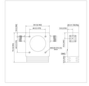
RF Solution offer a wide selection of Coaxial Isolator for global customers. UIYCI6075A is a Coaxial Isolator in Frequency Range of 45~270 MHz. It is made of high quality materials under a high standard, the Bandwidth Max of this product is 40%, Insertion Loss Max is 0.50~1.80 dB and Isolation Min is 18.0~25.0 dB. The component has a good working performance and stability, it is ideal for handling a Forward Power of 100/150/200 W.
