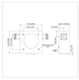
RF Solution offer a wide selection of Coaxial Isolator for global customers. UIYCI6060A is a Coaxial Isolator in Frequency Range of 45~270 MHz. It is made of high quality materials under a high standard, the Bandwidth Max of this product is 40%, Insertion Loss Max is 0.50~1.80 dB and Isolation Min is 18.0~25.0 dB. The component has a good working performance and stability, it is ideal for handling a Forward Power of 100/150/200 W.
