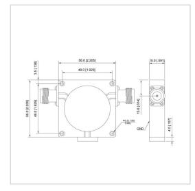
RF Solution offer a wide selection of Coaxial Isolator for global customers. UIYCI5656A is a Coaxial Isolator in Frequency Range of 130~900 MHz. It is made of high quality materials under a high standard, the Bandwidth Max of this product is 40%, Insertion Loss Max is 0.30~0.60 dB and Isolation Min is 15.0~23.0 dB. The component has a good working performance and stability, it is ideal for handling a Forward Power of 100/500 W.
