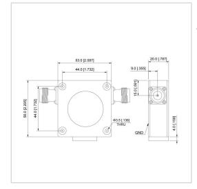
RF Solution offer a wide selection of Coaxial Isolator for global customers. UIYCI5356A is a Coaxial Isolator in Frequency Range of 300~1500 MHz. It is made of high quality materials under a high standard, the Bandwidth Max of this product is 18%, Insertion Loss Max is 0.20~0.5 dB and Isolation Min is 20.0~25.0 dB. The component has a good working performance and stability, it is ideal for handling a Forward Power of 300/500 W.
