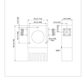
RF Solution offer a wide selection of Coaxial Isolator for global customers. UIYCI4580A is a Coaxial Isolator in Frequency Range of 250~1500 MHz. It is made of high quality materials under a high standard, the Bandwidth Max of this product is 30%, Insertion Loss Max is 0.25~0.70 dB and Isolation Min is 16.0~25.0 dB. The component has a good working performance and stability, it is ideal for handling a Forward Power of 100/300/400 W.
