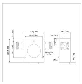
RF Solution offer a wide selection of Coaxial Isolator for global customers. UIYCI4550A is a Coaxial Isolator in Frequency Range of  $250\sim1500$  MHz. It is made of high quality materials under a high standard, the Bandwidth Max of this product is 30%, Insertion Loss Max is  $0.25\sim0.60$  dB and Isolation Min is  $16.0\sim25.0$  dB. The component has a good working performance and stability, it is ideal for handling a Forward Power of 100/300/400 W.
