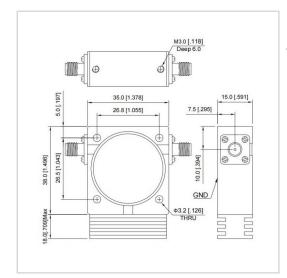
RF Solution offer a wide selection of Coaxial Isolator for global customers. UIYCI3556A is a Coaxial Isolator in Frequency Range of 200~1875 MHz. It is made of high quality materials under a high standard, the Bandwidth Max of this product is 100%, Insertion Loss Max is 0.20~0.65 dB and Isolation Min is 15.0~30.0 dB. The component has a good working performance and stability, it is ideal for handling a Forward Power of 100/300 W.
