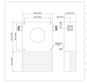
RF Solution offer a wide selection of Coaxial Isolator for global customers. UIYCI100166A is a Coaxial Isolator in Frequency Range of 70~130 MHz. It is made of high quality materials under a high standard, the Bandwidth Max of this product is 20%, Insertion Loss Max is 0.80~1.20 dB and Isolation Min is 16.0~17.0 dB. The component has a good working performance and stability, it is ideal for handling a Forward Power of 500 W.
