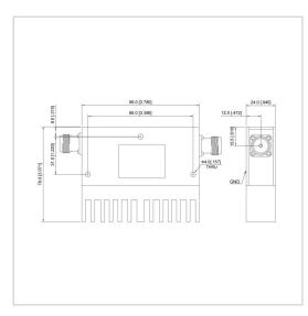
RF Solution offer a wide selection of Dual Junction Isolator for global customers. UIYCDI9678A is a Dual Junction Isolator in Frequency Range of 250~1300 MHz. It is made of high quality materials under a high standard, the Bandwidth Max of this product is 30%, Insertion Loss Max is 0.50~1.20 dB and Isolation Min is 32.0~50.0 dB. The component has a good working performance and stability, it is ideal for handling a Forward Power of 100/300/400 W.
